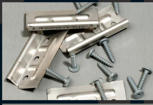
The clips are fixed to the substrate using two **Met-Seam®** grade 302 HQ stainless steel screws per clip. The clips are then concealed by the next consecutive panel thus hiding all fixings.
